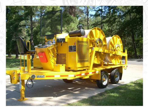
These four drum pullers with four separate pulling drums and ropes allow for the simultaneous or individual pulling in of three conductors and an earthwire.
