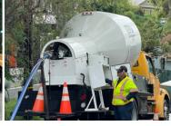
replacing the diesel engine power source with battery driven electric motors. We used the batteries and motors from the existing electric driven machines.
